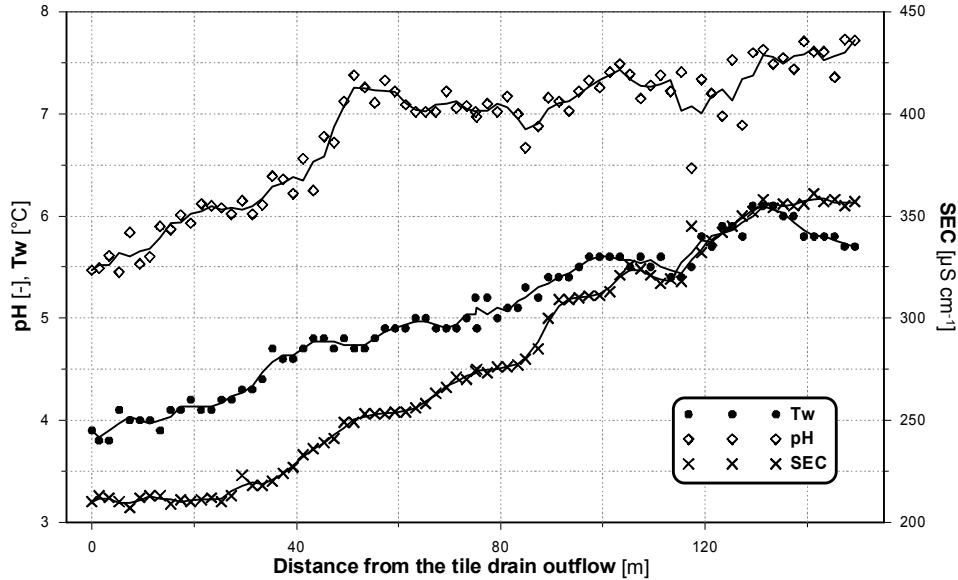
Fig. 4. Variations in water temperature ( T_w ), reaction (pH), and specific electric conductance (SEC) of river waters along the Radomyski Potok channel on March 5 th , 1992. Lines denote a three-element moving average. Obr. 4. Priebeh teploty ( T_w ), pH, a mernej elektrickej vodivosti (SEC) vody v rieke pozdĺž toku Radomyského potoka 5. 3. 1992; čiary označujú kľzavý priemer.
